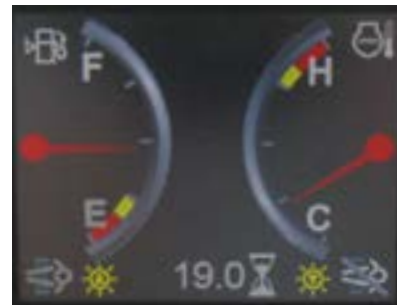
Digital color display This information center shows real time fuel consumption, engine rpm, machine hours, engine diagnostic codes, warning indicators and much more. Models 1350 R, 1500 R & 1650 R
