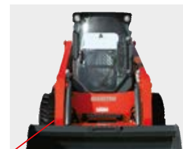
● Over-the-tire Design provides wider access and improved visibility. Models 2200 R and 2600 R
