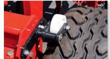
▲ -Driving wheel brake. / Frein de la roue motrice.
