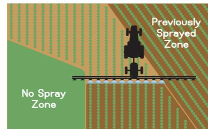
**Individual boom section control** gives you the most accurate and cost-efficient system possible—automatically avoiding no-spray zones and previously sprayed areas. With AccuBoom, you spray only where you want to spray. No more, no less.
