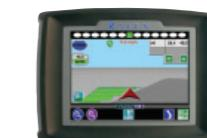
**Envizio Pro:** Integrated 10Hz DGPS receiver with sub-meter accuracy, two-product capability, optional single-product VRA, 6.4-inch touch-screen display, and wireless capability. Scalable.
