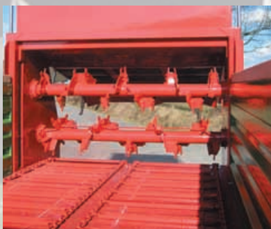
High performance spreading system: two horizontal rotors with aggressive welded-on shredder tines face-hardened for long working life
