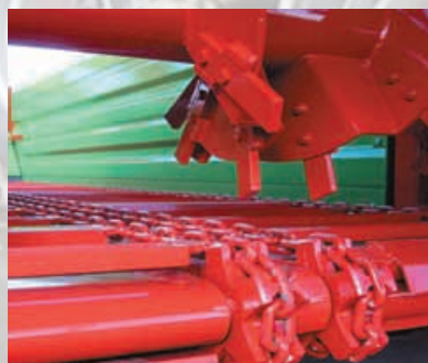
Floor scraper with four strong chains and spreader system are optimally matched with one another
