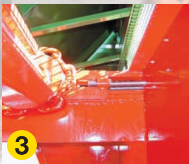
3 Screw tensioners for the floor scraper system. Every chain can be individually tensioned
