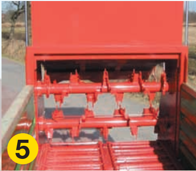
5 Two horizontal spreading rotors, regulating gate completely open, hydraulic rear gate open and floor scraper with four high strength tempered chains
