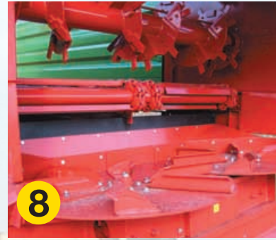
8 Broadcaster discs with six adjustable thrower blades, replaceable throw-direction guards of Hardox steel (standard)
