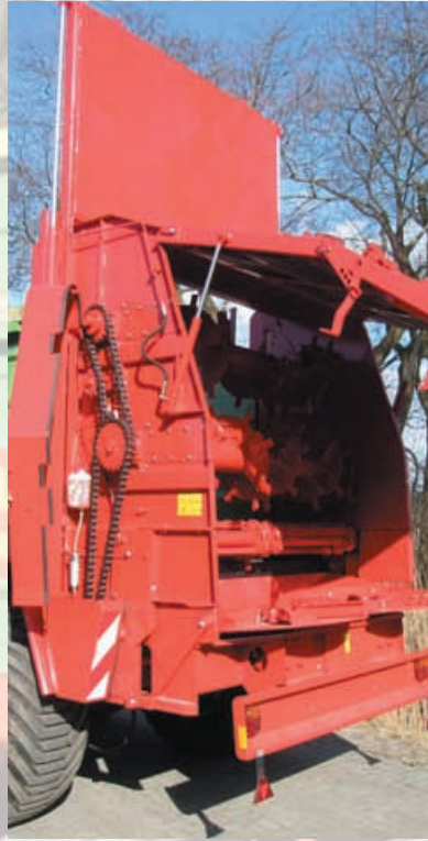
Spreader rotor drive via 1.25 inch chains
