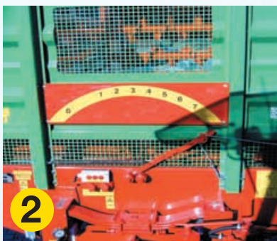
2 Indicator showing regulating gate height, drawbar suspension and transparent front trailer wall with view through to spreader
