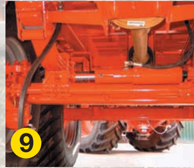
9 Following steering axles with weight-dependant steering system: the heavier the weight the more consistent the straight line progress
