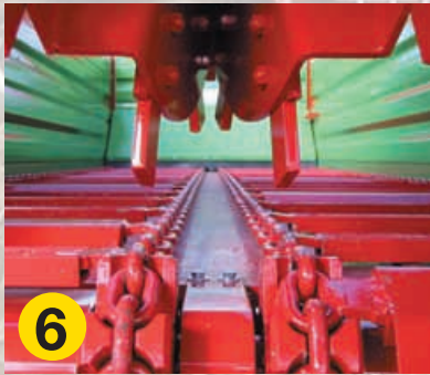
6 Four 14 mm floor scraper chains with large links giving high self-cleaning efficiency and long working life
