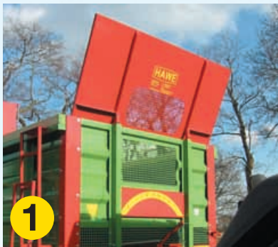
1 Protective metal grill in front, transparent front wall and folding ladder to the right of drive direction
