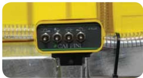
“**Elektrooil**”: Control box for the boom movements by electro valves. This requires one double acting valve.
