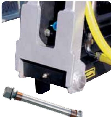
All boom joints are constructed with steel pins and self-lubricating bushings.
