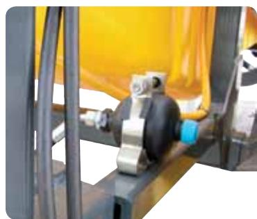
"Soft Damp" Hydraulic circuit with nitrogen bowl for the correct damping of the boom.
