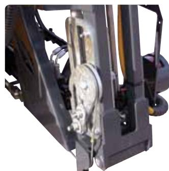
The new automatic blocking of the equalizer allows folding and unfolding of the booms preventing the opened side going down so maintaining the boom ride height.
