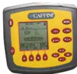
Computer “**COMPACT**” for the automatic spraying control showing
