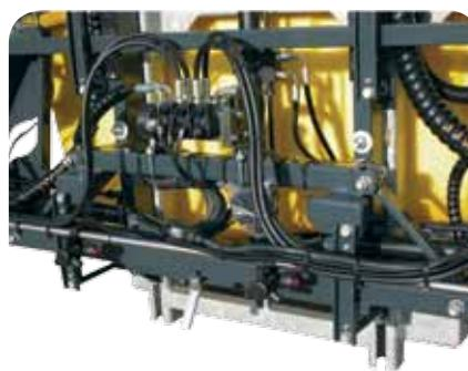
The efficient trapezoidal equalizer allows through connecting rods and sliding shoes an optimal parallelism of the boom with the ground.
