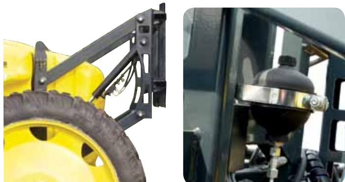
"Quadrilever" pantograph lifting system of the boom with parallelogram by 2 hydraulic cylinders. It is all aided by a hydro-pneumatic system with nitrogen bowls. The joints of the lifting device are realised with self-lubricating pins and adjusted steel pins. The "QUADRILEVER" system assures great stability for the boom, both during treatment and during transfer, also allowing greater extension in height compared to classic vertical lifting mast.
