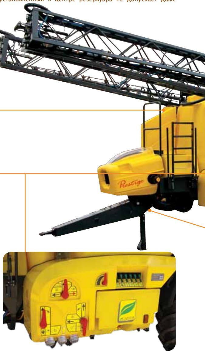
**“Hub Service”:** work station for preparation of spraying treatments. All operations can be carried out in the same place thanks to multi-purpose valves for: checking of the loading, return, system and tank washing phases. Their activation is guided by coloured pictograms.
