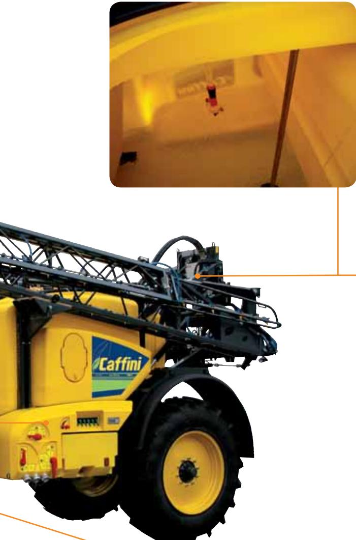
**"Robot-jets"**: thanks to these rotating nozzles working with high pressure clean water, excellent washing of the tank walls is assured.
