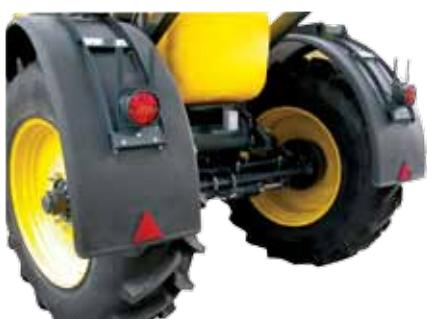
**"Trackmatic Profi"**: Steering system managed through information received by an electronic gyroscope placed on the tractor. The hydraulic steering of the wheels is automatically. "Trackmatic Profi" performs two functions:
