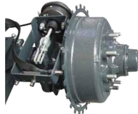
**Brakes:** these are available in hydraulic or pneumatic, with manual control or automatic with the tractor pedal. Road regulations of 25km/h or 40 km/h or 50 km/h (Germany).
