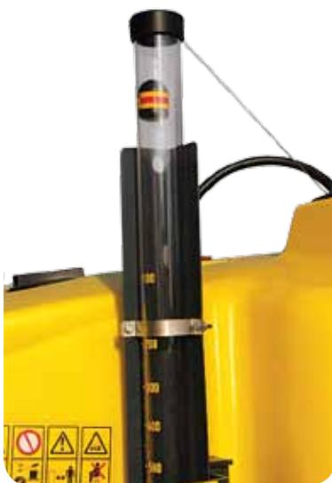
The “dry-type level gauge” (without contact with tank liquid) is visible from the tractor and from the filling side, for an easy read of the liquid quantity inside the tank. The feeder, which is positioned in the middle of the tank, is less affected by sprayer chassis uneven standing.
