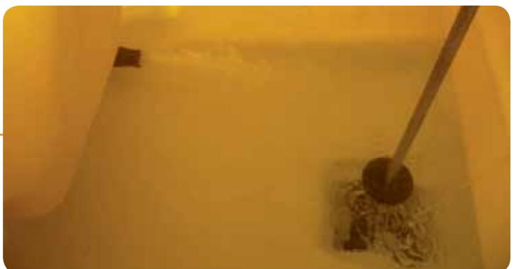
The powerful mixing system guarantees homogeneity of the mix inside the tank. The intensity of the mix can be adjusted to avoid excessive forming of foam.
