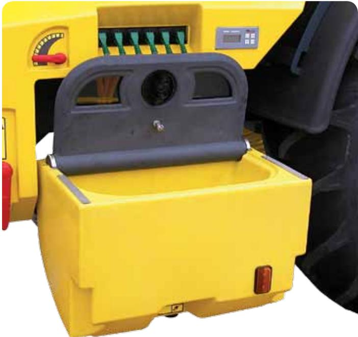
The plant protection products are quickly dissolved inside the “Premixer” thanks to special nozzles working at high pressure. Once ready, they are incorporated inside the tank with a powerful water-injector, avoiding any contact with the operator. The Premixer hopper is equipped with a rotary container-washing jet with which it is possible to fully rinse containers prior to safe disposal.
