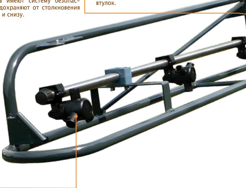
The nozzles and tips are protected inside the boom structure in order to avoid any contact with the ground or obstacles. The pipes are in stainless steel. The optional "trijet, quadrijet or pentajet" nozzles are fitted with anti-dripping membrane device, shutdown position and the ring nuts are of the "quick coupling type".
