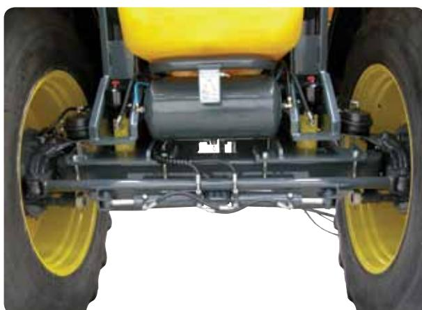
**Suspensions**: an effective and innovating hydro-pneumatic system consisting of two cylinders operated by a nitrogen accumulator gearbox assures a best dampening of the sprayer both in empty and full load conditions, as well as higher spraying and transfer speeds. This system in combination with the other available damping systems, protects also the frame, boom and tank unit.
