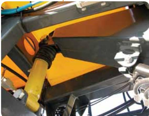
**Drawbar with suspension:** the sturdy drawbar is available also damped by an hydraulic cylinder and nitrogen bowl. With the drawbar damped it's possible to obtain great advantages as the stability during transfers avoiding swinging of the sprayer and increasing the boom's stability during the spraying.
