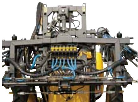
The stability of the boom is guaranteed from equalizer with oscillating pendulum system. This assures an optimal parallelism with the ground for a better quality of spraying. The new dampers with adjustable multi-layer connecting rods guarantee the damping. All the sprayers are standard equipped with a hydraulic trim control allowing the boom to adapt itself to sloping terrain.
