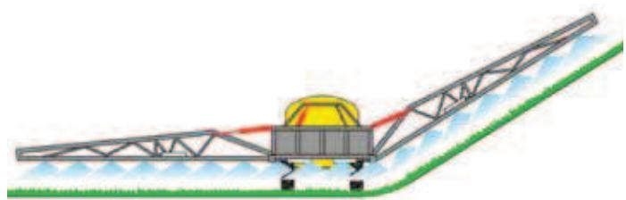
**Variable Geometry** independent right and left. The system includes nitrogen bowls for the boom damping on both sides.
