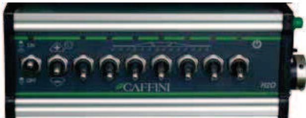
**"Elettrocontrol"**: a block of 5/7/9 electric motor valves for the section of the boom. This block also has an electric valve for general closing (by pass) and electric adjustment of the pressure. The functionality of the electric distributor is guaranteed from a practical self-cleaning filter.
