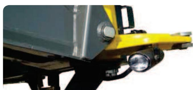
**Set night-work lights:** positioned in the centre of the bar, these special long beam lights enable visibility of the nozzles during night-time treatments.
