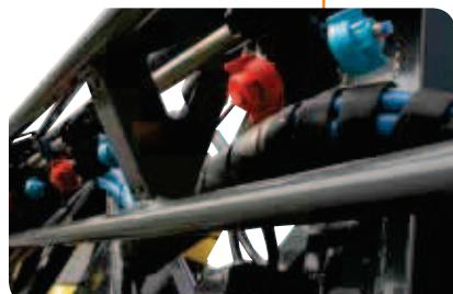
**The nozzles and tips are protected** inside the boom structure in order to avoid any contact with the ground or obstacles. The pipes are in stainless steel. The optional "trijet, quadrijet or pentajet" nozzles are fitted with anti-dripping membrane device, shutdown position and the ring nuts are of the "quick coupling type".
