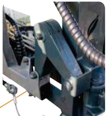
**The new suspensions** (boom H.B.L.) with adjustable multi-layer connecting rods in steel and Teflon assure an excellent damping of oscillations.
