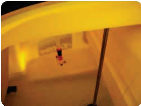
**"Robot-jets"**: thanks to these rotating nozzles working with high pressure clean water, excellent washing of the tank walls is assured.
