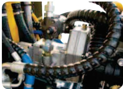
The fan can be actioned directly by the hydraulic pump of the tractor (the system requires 55 l/min) or by an independent system (look at the picture) actioned by the cardan shaft together with the pump of the sprayer. The system is consisting of: hydraulic pump, oil tank with filter and outside level gauge.
