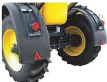
**"Trackmatic Profi"**: Steering system managed through information received by an electronic gyroscope placed on the tractor. The hydraulic steering of the wheels is automatically. "Trackmatic Profi" performs two functions:
