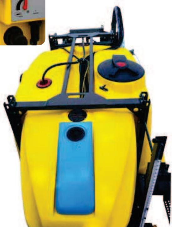
The powerful mixing system guarantees homogeneity of the mix inside the tank. The intensity of the mix can be adjusted to avoid excessive forming of foam.
