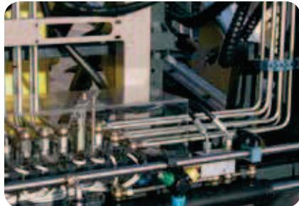
The bulk of pipes for distribution are made of stainless steel, therefore are free from breakdowns and maintenance.
