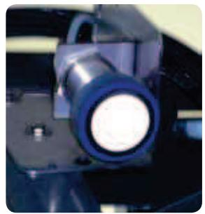
**"Trailmatic"**: Steering draw bar with electronic control by a sensor connected to the towing hook. It allows through a system composed by cylinder, electric valves and special software, following the tractor tracks.
