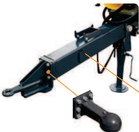
The "Prestige" range comes fully equipped with fixed drawbar adjustable in height with towing eye. The ball attachment is an optional extra. For an easy tractor coupling is provided a sturdy servo-steering.
