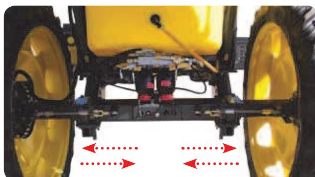
Standard manually adjustable track 1.800 to 2.250 mm (2.200-2.800-3.300 l)
