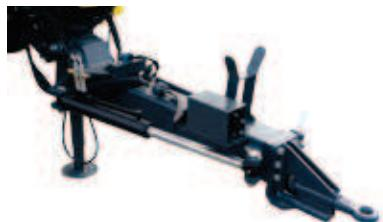
Hydraulically activated steering drawbar. Compatible for "Trilmatic & Trilmatic Profi" electronics management.
